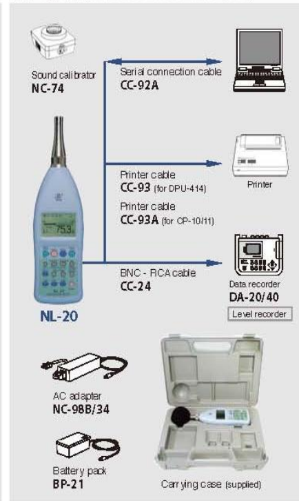
System diagram NL-20 (Equipment other than sound level meter is optional)
