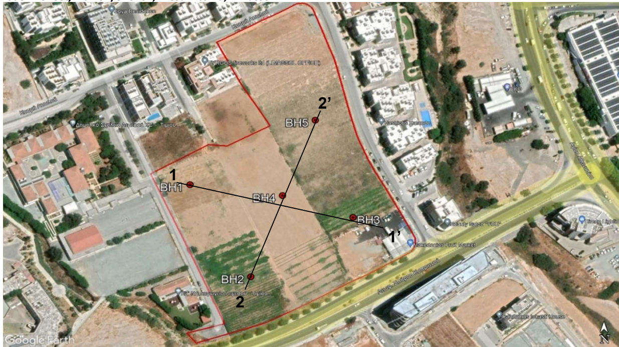
Figure 6. Boreholes' and Cross Sections' locations
