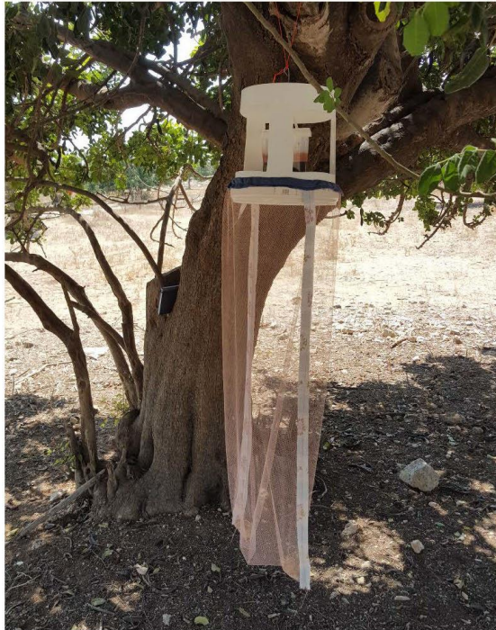
Figure 2. Wine trap used to attract and live-trap any P. b. cypricus from the study-site.
