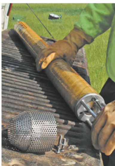
Picture 8: Automatic pneumatic submersible recovery pumps and operational principal
